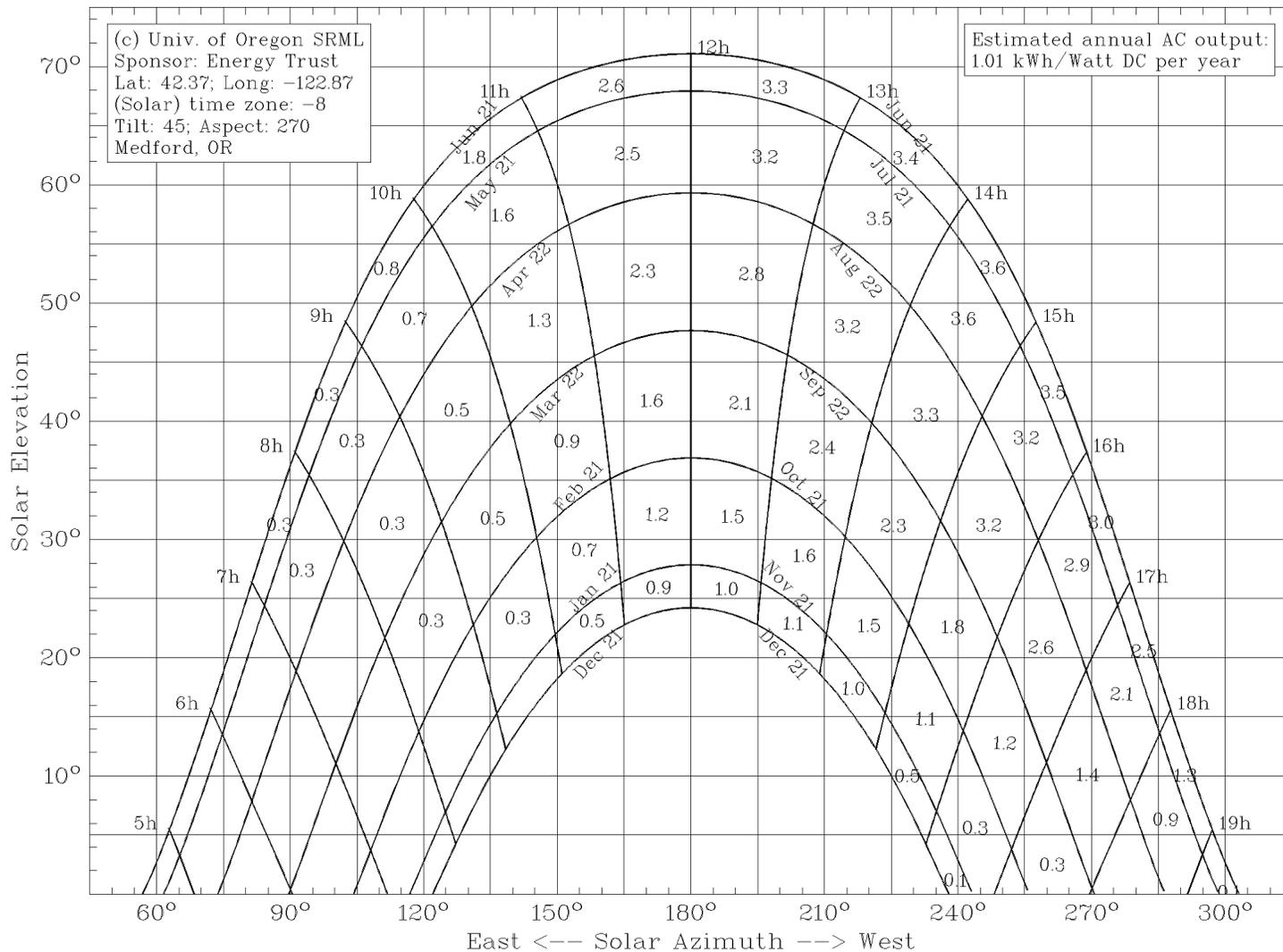
Draw the horizon on the sun path chart and shade obstructed areas. To calculate the percent reduction due to shading, enter the percentage of system power output shown on the sun path chart for areas shaded by obstructions into the table on the right.
