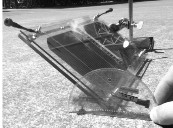
Fig. 6.2: Using a protractor to measure the tilt of the cells.
