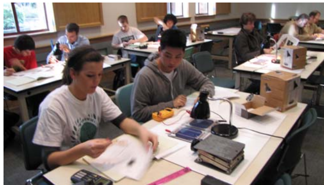
Fig. 9: Students in a freshman physics seminar are measuring the DC current with the lamp at different heights from the solar cells.
