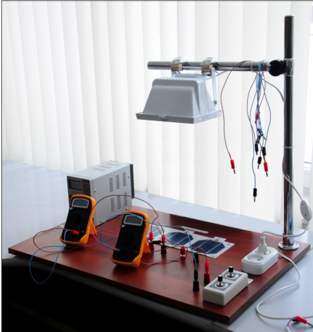
Fig. 1: Russian PV lab kit for study characteristics and parameters of solar cells also principles of solar module' design.
