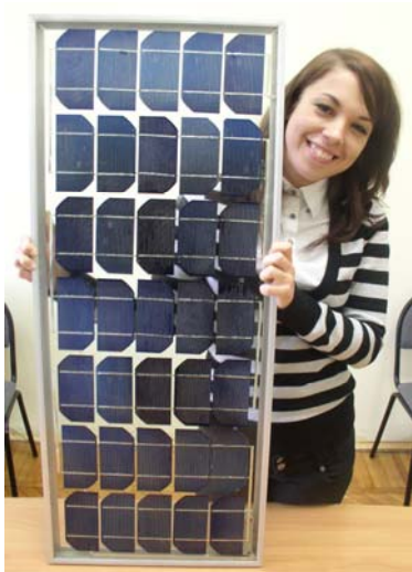
Fig.10. Plastic free 20 W module of full size with mono-crystalline solar cells.
