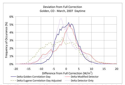
Fig. 7. Distribution of the difference between the full correction model IR radiative loss values during the day from those of other models under study. Data from SRRL in March, 2007. Plot represents over 20,000 one minute data points divided into 0.5 W/m<sup>2</sup> bins.
