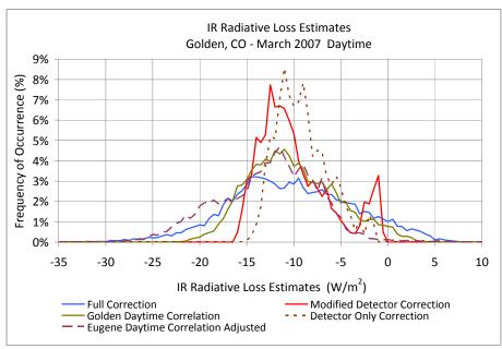
Fig. 6. Distribution of IR radiative loss values during the day from the models under study. The data are from SRRL in March, 2007. The plot represents over 20,000 one minute data points divided into 0.5 W/m2 bins.
