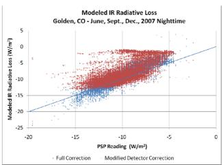
Fig. 2. Comparison between the full correction and the modificed detector correction for the IR radiative losses during the night. By measuring the pyranometer's IR responsivity, an improvement in the estimated IR radiative loss can be achieved. While the difference at higher IR radiative loss values is smaller, it still exists. In addition there is a shift of many points to low estimated IR radiative loss values. The reason for this shift should be investigated.
